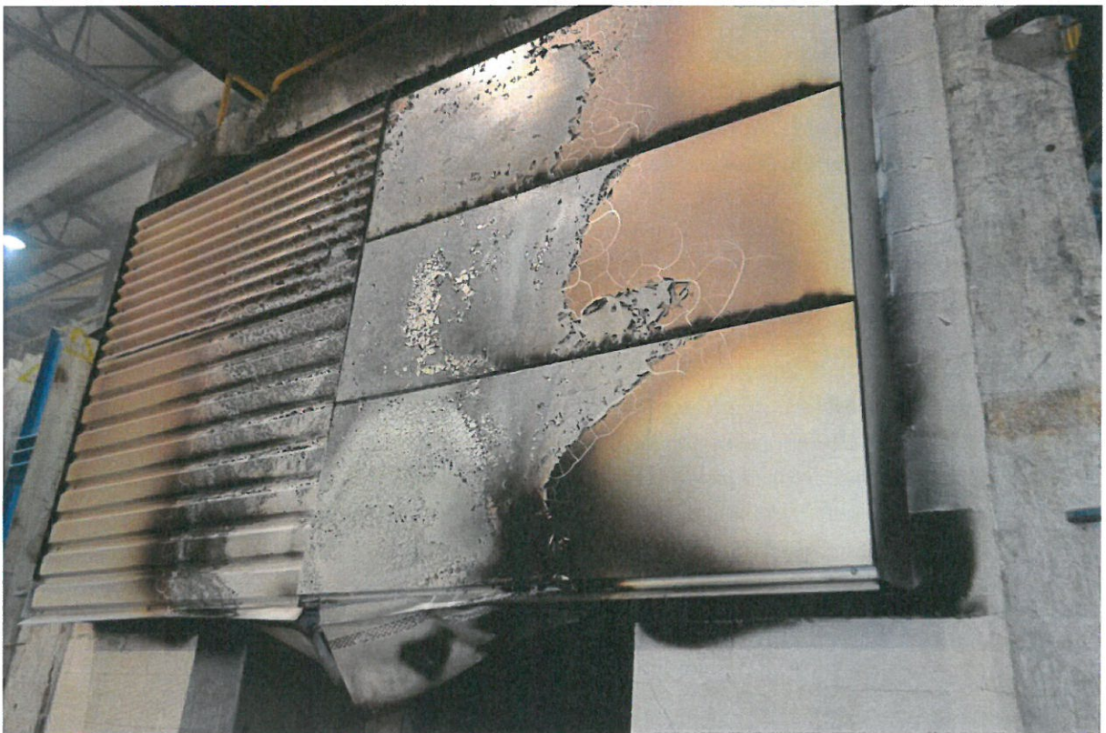
Fig. 44. Test specimen after the test
