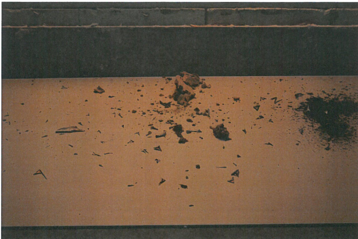
Fig. 33. Fragments of mineral wool that have fallen off, t = 43 min
