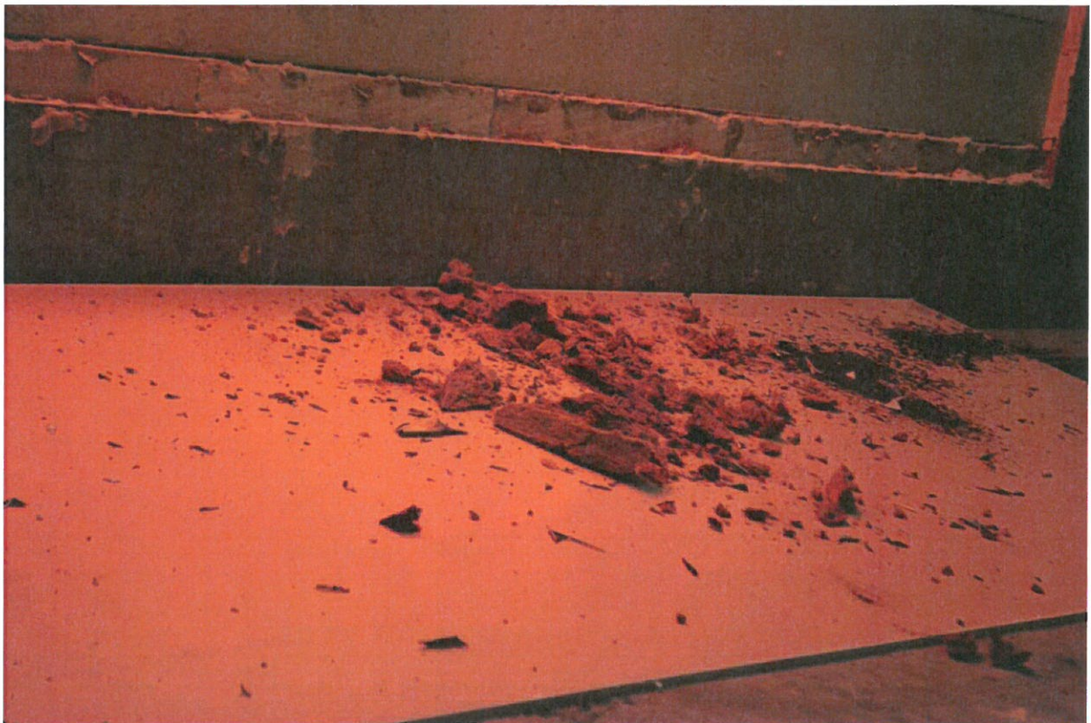
Fig. 38. Fragments of mineral wool that have fallen off, t = 100 min.
