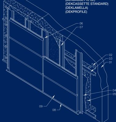
An integral form part of the DEKMETAL facade system form also the additional elements without static functions. It's all about corners cover profiles, steel lining, flashing of attic, weather moldings, ventilation grills, etc. These elements may vary in format according to customer's requirements.
